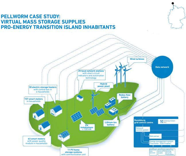
The island of Pellworm located in the North Sea belongs to the most sunny and windy regions in Germany. Wind power installations and continuously improving solar panels have been used here since the 1980s. Now they produce a total of 20 million kWh of electricity per year. That is far more than the 1,000 island residents consume. Nevertheless, electricity is also imported from the mainland at times.
