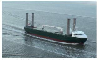
Enercon GmbH's E-Ship 1 transports wind turbines with the assistance of the wind on the high sea
