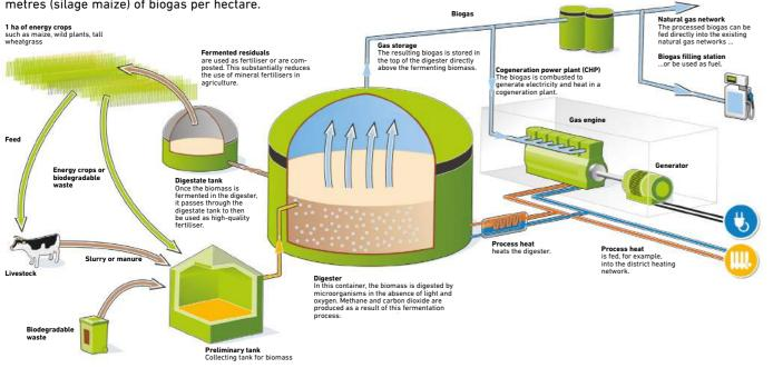
The methane content of the biogas is increased to adapt it to
