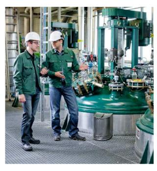
Staff check the esterification reactors, which are used for the production of biodiesel
