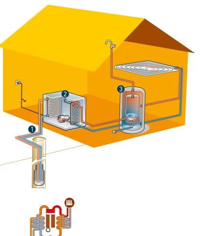
The electric compressor in the heat pump compresses the vapour. This in turn increases its temperature. The heat can then be used for space and water heating.
