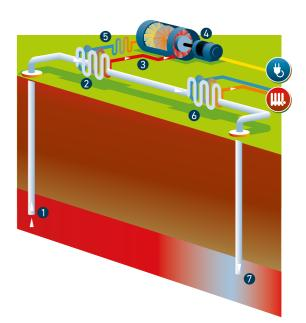
From depths of 2,000 to 4,000 metres, **1** thermal water at a temperature between 90 and 150 °C is pumped to the surface.
