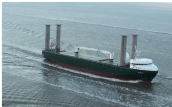
Enercon GmbH's E-Ship 1 transports wind turbines with the assistance of the wind on the high seas.
