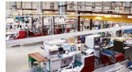
The medium-sized printing company August Koopmann GmbH from Stuhr (Lower Saxony) had the lighting of its 3,500-m<sup>2</sup> production hall converted entirely to LED: 800 existing systems with fluorescent tubes were replaced with 350 new systems using highly efficient LED technology to now efficiently and economically illuminate machines, work stations and storage facilities.
