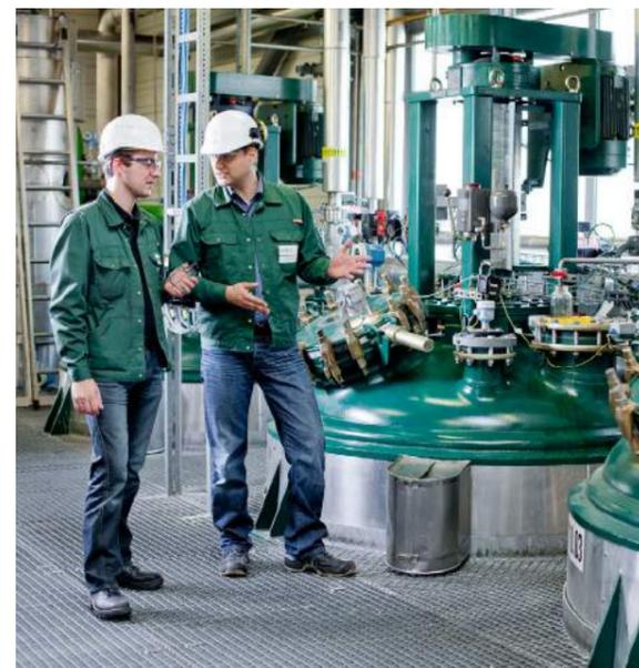
Staff check the esterification reactors, which are used for the production of biodiesel.
